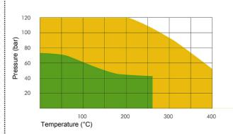
The P x T diagram above indicates the service limits for **NA-1100** considering the simultaneous influence of pressure and temperature (chemical suitability assumed). The green area represents the normal service limits, while the orange colored area shows the maximum application limits. For those cases, please consult our technical department.
