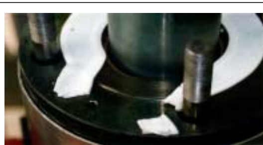
HOBT rig – PTFE Gasket Blow Out example
