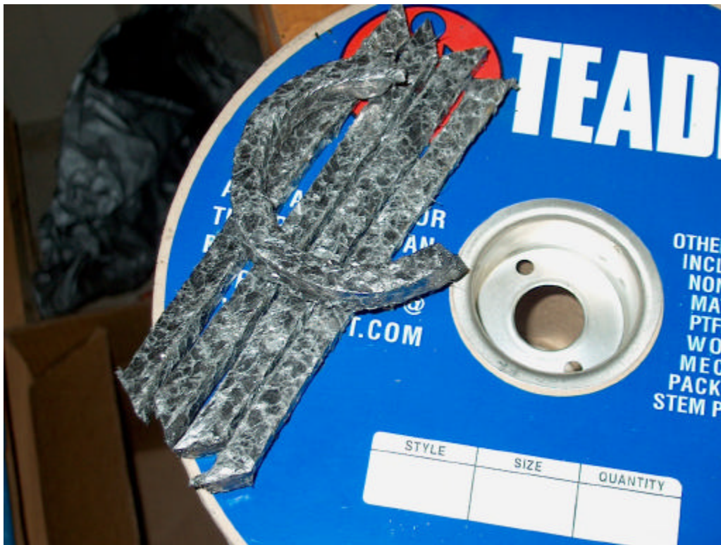
Packing received from manufacturer. Five rings cut at 45 deg. angle.
