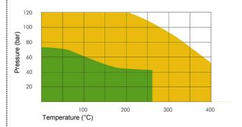
The P x T diagram above indicates the service limits for NA-1100 considering the simultaneous influence of pressure and temperature (chemical suitability assumed). The green area represents the normal service limits, while the orange colored area shows the maximum application limits. For those cases, please consult our technical department.
