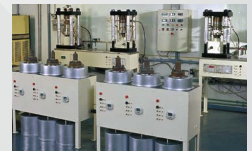
50-T Gasket Test Bench
