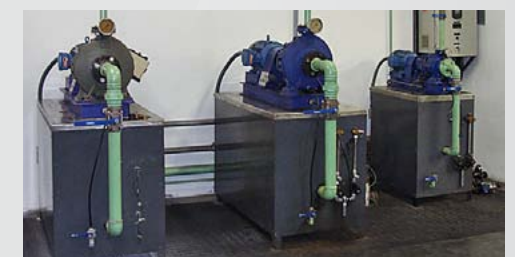
Pump Test Stand for evaluation of packing performance
